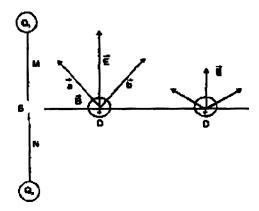
When a spark passes across S, stream of electrons pass across the spark gap from the negatively charged sphere to the positively charged sphere, reversing their polarities. In this situation the direction of the electric field at C and D will be reversed. Thus, at each passage of spark the polarity of charges on Q<sup>1</sup> and Q<sup>2</sup> reverses and the electric field direction in the surrounding region also reverses; i.e. the electric field oscillates.
