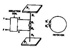
**Explanation**. The high potential difference across the metal plates ionizes the air between the spheres  $S^1$  and  $S^2$  and allows a path for discharge of plates. During the discharge of plats, a spark is produced between the spheres due to the high potential difference.
