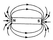
by a current carrying straight solenoid is identical to that produced by a bar magnet. The magnetic field lines do not exist in reality. This hypothetical concept has been developed in order to visualize the strength of magnetic field in different regions and the effect of magnetic field. The regions, where the magnetic field lines are close enough (crowded), the magnetic field is considered as quite strong there.
