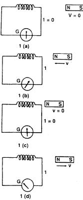
whenever, the coil and the magnet are stationary with respect to each other, no deflection is observed.
