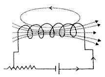
The parameter L (i.e., total flux due to unit current) here is called the self-inductance of the coil. Its value depends upon the size and shape of the coil as well as the number of turns. It also depends upon the magnetic property of the medium of the space within the coil, e.g., if the coil is wound around a soft iron core (after ensuring proper insulation) it attains a very large value.
